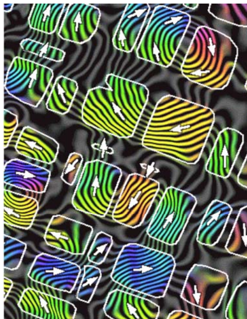
Fig. 1. Electron holography image revealing the complex magnetic microstructure of an array of ~ 100 nm sized cubes of magnetite (Ref. 1).
