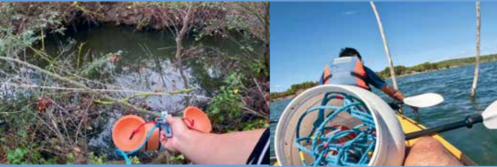
Left: Gio using a depth sampler to get access to water in the river. Right: Lin sampling the salinity in the lagoon, in the Balaruc Le Vieux.
