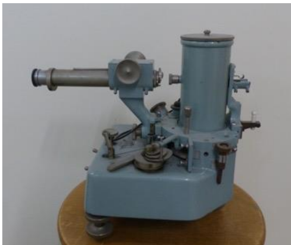
Figure 1. A Unicam single crystal rotation and oscillation X-ray camera from the X-ray lab in the Department of Earth Sciences. It is an original instrument inherited from the Dept. of
