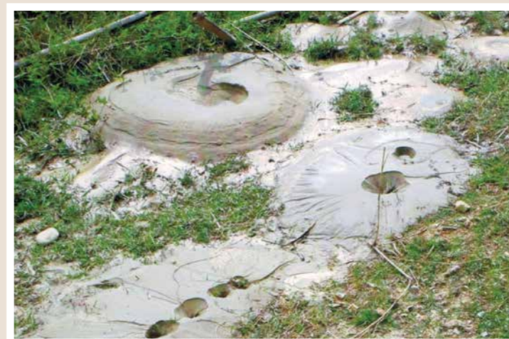
FIG. 11 Liquefaction caused by the 2011 M5.8 Yingjiang earthquake in Yunnan province, China, as evidenced by sand boils
