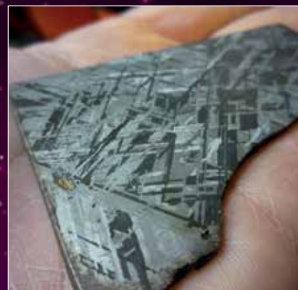
Polished and etched sample of an Fe-Ni meteorite showing the familiar Widmanstätten pattern.
