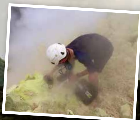
Left: Dr Brendan McCormick Kilbride deploys a MultiGAS analyser to measure the chemical composition of volcanic gases.
