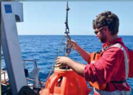
Left: Tim Greenfield overhauls the ocean-bottom seismometer before the deployment.
